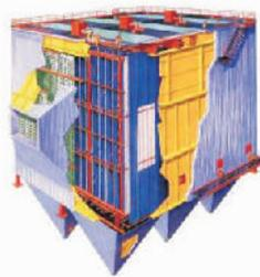
Gambar 2.1 Electrostatic Precipitator
